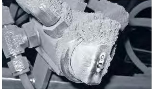
The air cap of two-substance nozzle with horns shows the typical product build-up (bearding). This clogs the air ducts and impairs the spraying pattern. The SCHLICK ABC cap, however, does not experience any product build-up at the nozzle orifices and thus allows for an optimal spraying pattern.
