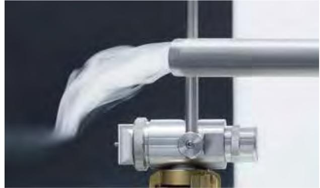
A comparison of the flow patterns reveals that the dust particle flow – simulated here in the form of fog – stays away from the anti-bearding cap much better than it does from the conventional flat spray cap. The ABC cap thus counteracts the conventional bearding effect.
